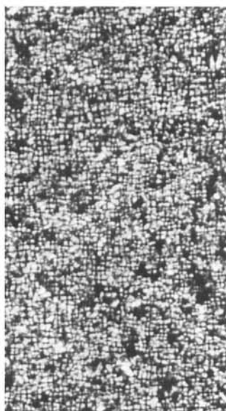
FIGURE 3. Cholesteric non-planar texture with focal conics of sample P4 at 110°C. (See Color Plate VIII)
